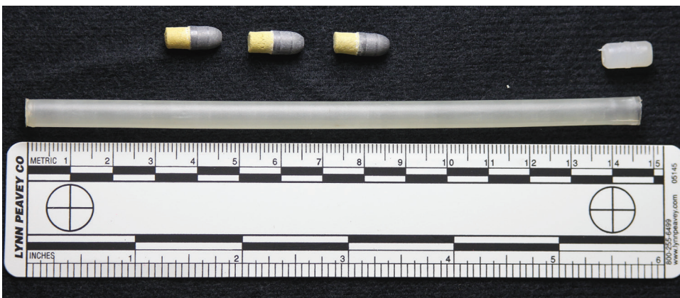
Figure 2.10 Daisy V/L caseless cartridges. The bare lead projectile is seated against the yellowish, granular propellant charge. The plastic tube is the container the cartridges were shipped in. (Image from author's collection.)
